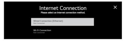
If the network is not configured for DHCP, or if you want to enable/disable IPv6, specify static IP configuration data (applicable only for IPv4), or change the network configuration from Manual to Automatic, select Wired Connection (Ethernet) and press OK.
