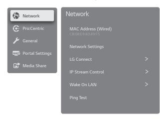
Use the Up/Down arrow keys on the Installer Remote to select the desired menu option and then press **OK**. Refer to the following sections for information on each of the IP Environment setup options.
